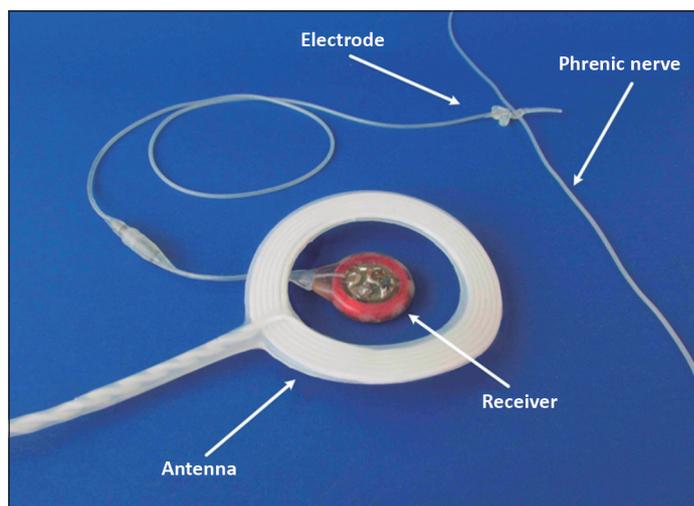
**Figure 1.** Components of the diaphragmatic pacemaker and schematization of the contact of the electrode with phrenic nerve.
